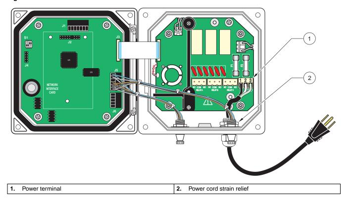
Figure 3-16 Local Disconnect for Hard-wired Line Power
